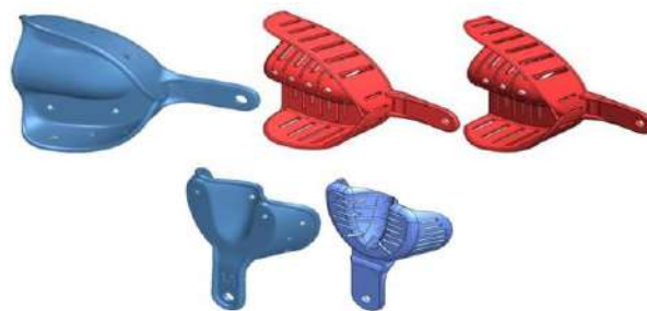
Figure 13. Scanned spoons U1 and U4 and redesign of the spoon
