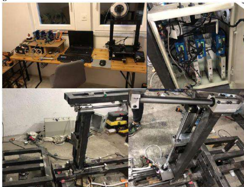
Figure 6. Equipment testing and software development (upper left), control unit assembling and wiring (upper right), machine assembling (bottom left and right)
