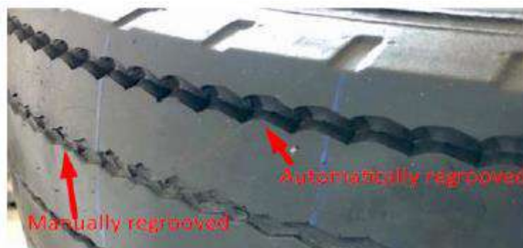
Figure 15. Comparison between manual and automated regrooving processes
