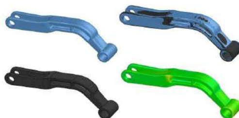
Figure 14. Reverse engineering on a lever
