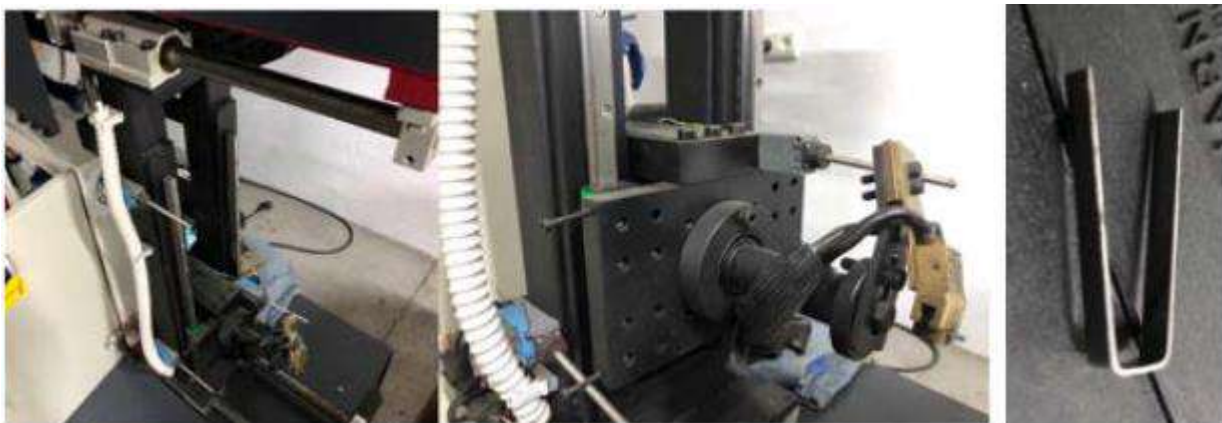
Figure 9. Mechanism for manipulating the regrooving tool (left), the regrooving tool (middle), the regrooving blade (right)
