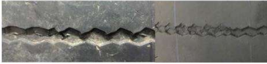
Figure 3. Poorly regrooved tire using manual regrooving tool
