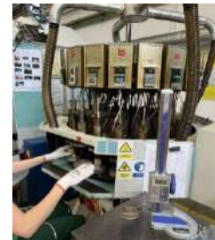
Figure 5. Circular press for pressing and sealing filters
