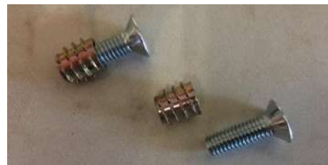
Fig.15: Countersunk screw M8x25 with internal / external threaded nut
